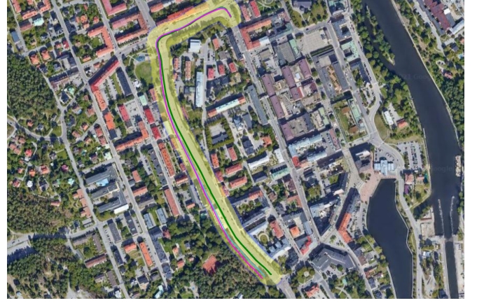
Fig. 5. Results of the odometry estimation from L_F (blue) and L_R (magenta) lidars plotted in Google Maps with respect to the GT (green) with initial calibration parameters. The GT was generated using Novatel GNSS.
