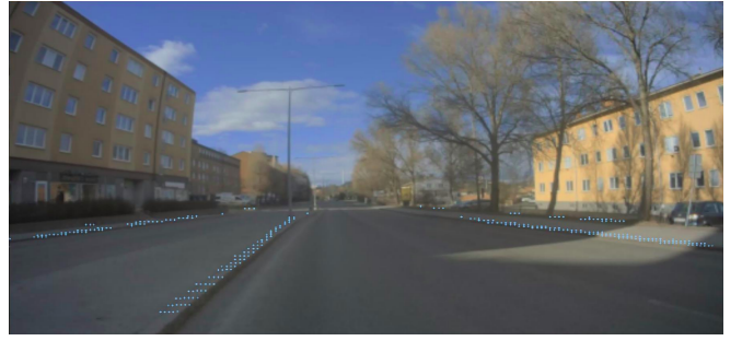
Fig. 9. Lidar point cloud projected into camera perspective with filtered curb semantics, shown as cyan colored points.
