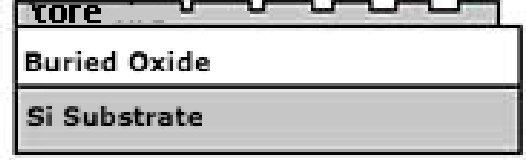
(b) Apodized grating coupler cross-section
